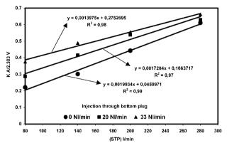
6 Lumped kinetic parameter KA/(2·303 V) (where K is mass transfer coefficient, A is liquid/gas interfacial area, V is volume of liquid) versus gas flowrate with and without gas injection through porous plug: x axis is for gas injection through upleg only
