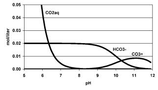
3 Equilibria between species in sodium hydroxide solution ([NaOH]=0.02 M) and gas phase containing CO<sub>2</sub>
