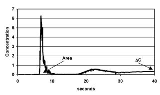
2 Typical concentration-time curve for calculation of circulation rate: (A: area under first peak, ΔC: difference between final concentration and initial concentration of tracer)
