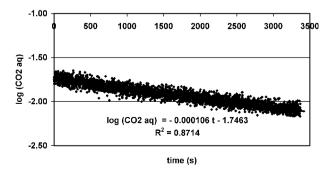
4 Kinetics of CO<sub>2</sub> desorption from NaOH solution
