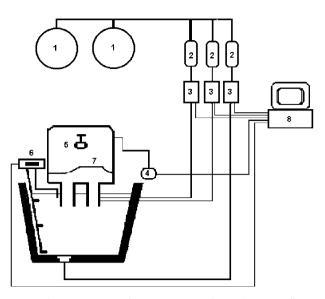
1: air compressor; 2: pressure regulator; 3: mass flowmeter; 4: pressure transducer; 5: to vacuum pump; 6: conductivity meter; 7: injection point; 8: PC and A/D board
