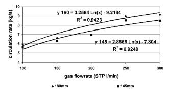
8 Liquid circulation rate versus gas flowrate for two downleg diameters 180 and 145 mm: upleg diameter is kept at 145 mm
