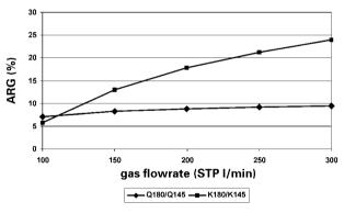
10 Circulation average relative gain (ARG) (Q180/Q145) and degasification ARG (K180/K145) as function of gas flowrate for two downleg diameters 180 and 145 mm
