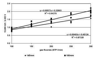
9 Lumped kinetic parameter versus gas flowrate for two downleg diameters 180 and 145 mm: upleg diameter is kept at 145 mm
